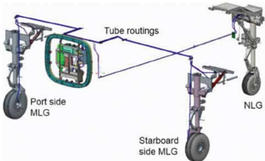
Landing gear system for Tapas UAV
