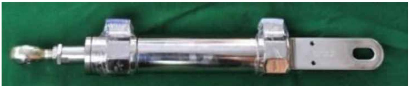
RLG Retraction actuator of Tapas UAV
