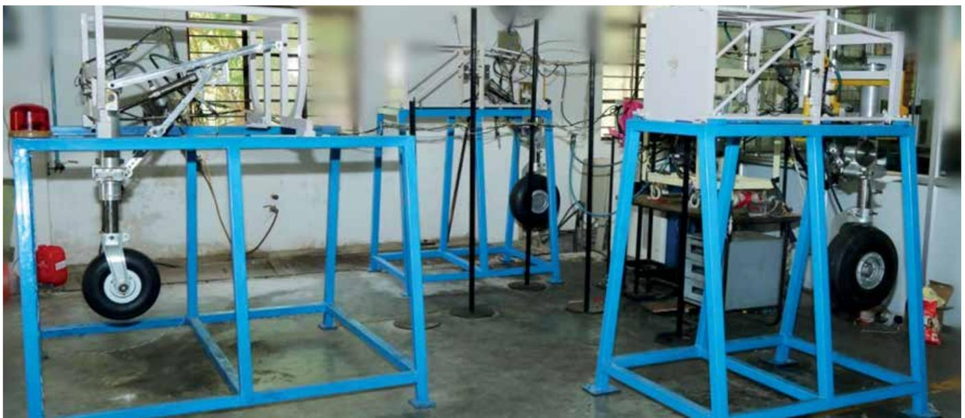
Testing of LGS in Integration Test Rig
