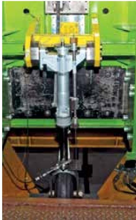
Landing gear spring curve test
