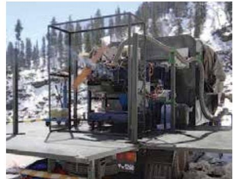
Turbo charged EFI engine on mobile test platform at Manali (6,752 ft)
