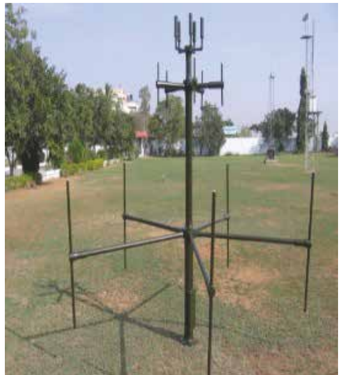
DF Antenna sub system for COMINT
