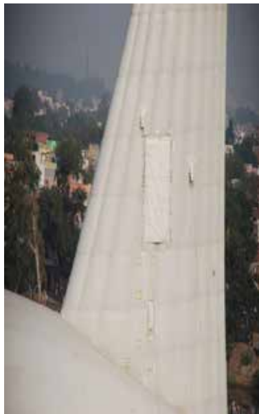
Conformal Printed Antennas on Tail of Aerostat
