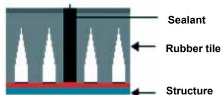
Sealant used for sealing the gap between rubber tiles
