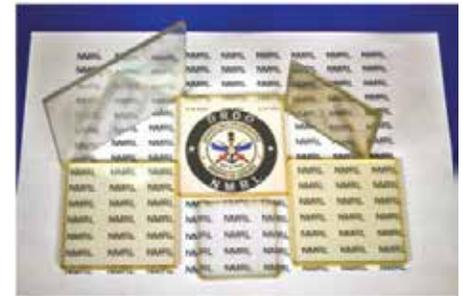
Transparent polycrystalline spinel ceramic tiles of up to 4 inch x 4 inch dimension
