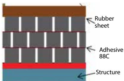
**Schematic of the application of NMR51K and NMR88C adhesives**
