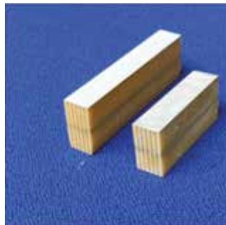
2-element Piezocomposite stacks for receiver and projector transducer arrays of Portable Diver Detection Sonar
