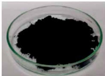
Corrosion resistant catalyst for PAFC
