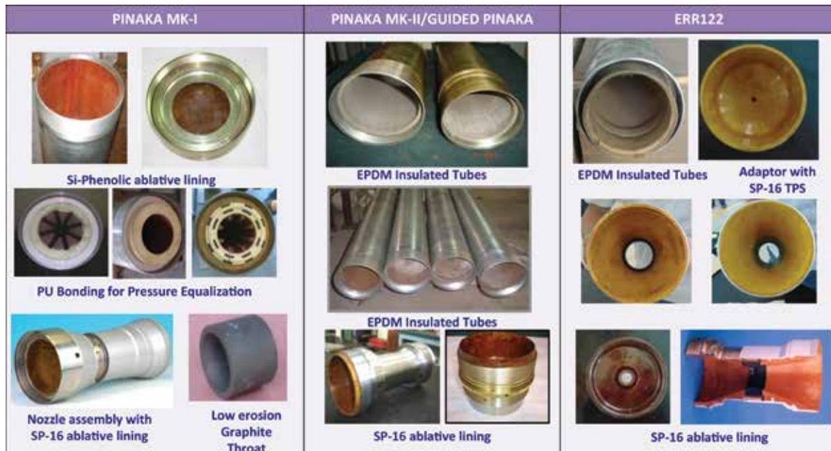
**Thermal Protection System used for Rockets**
