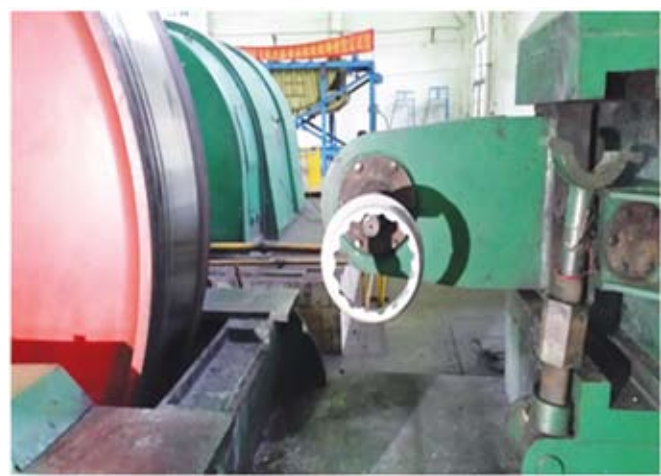
Typical Tyre Dynamometer for Aviation Requirements
