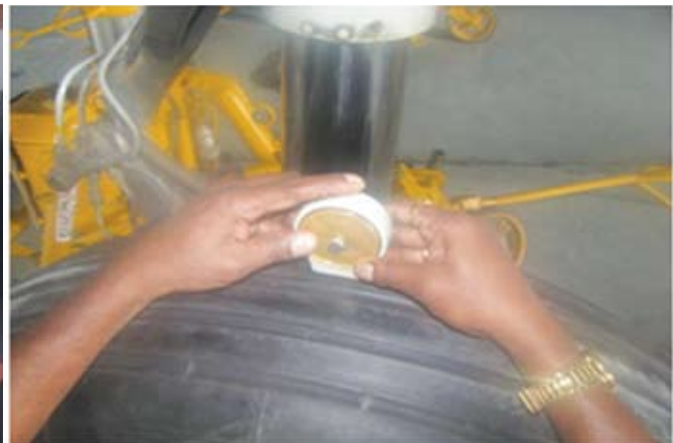
Tyre Pressure Test Under Progress
