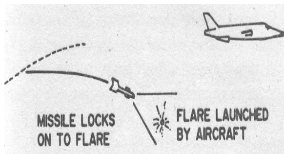
Most dispensers used for chaff can also be used to drop infrared flares capable of confusing heat-seeking missiles. In addition to protecting tactical aircraft, flares also play a role in protecting strategic bombers. Early infrared (IR) weapons were very vulnerable to decoy flares, but most recent designs use flares or dual operating frequencies in order to estimate roughly where the peak level of IR output lies.
