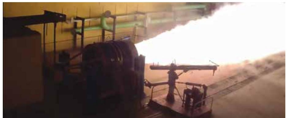
The 33T class (Thrust) solid rocket motor is one of the largest rocket motors with HD1.1 class of propellant in a composite casing being processed in India. The static testing of the motor involved data acquisition of 30 channels for temperature, 36 channels for strain, 2 channels
