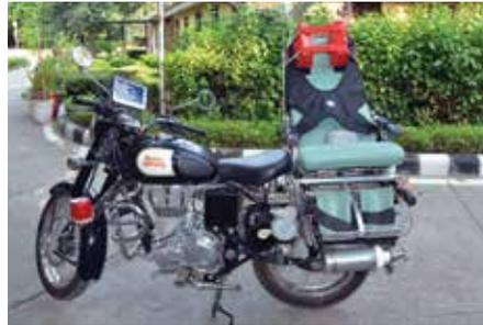
from low intensity conflict areas. This will be handy in the congested streets and remote locations, where access through ambulance is difficult and time consuming. The bike can respond to a medical emergency faster than a four-wheeler due to its functionality and integrated emergency medical support system. Rakshita is fitted with a customized reclining
