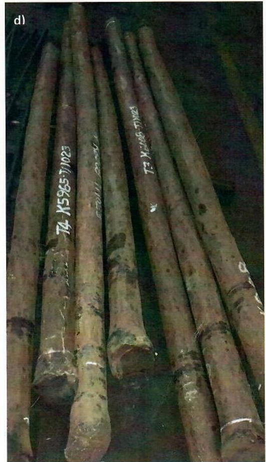
Figure-1 a) 1.4 T electrode prepared by plasma welding of compacts. b) Machining of secondary ingot before forging c) Forging of ingot in 1500 T press d) 120 mm dia intermediate billets for producing 100 mm dia finish product
