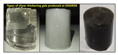
Prototype of flexible STG filled laminates have been prepared and tested for ballistic impact applications. The shear thickening mechanism resulted to efficient dissipation of energy by rearrangement of functional nanofillers due to squeezing out of polymeric matrix from the nanoparticle agglomerates which ultimately resulted into thickening of gel.
