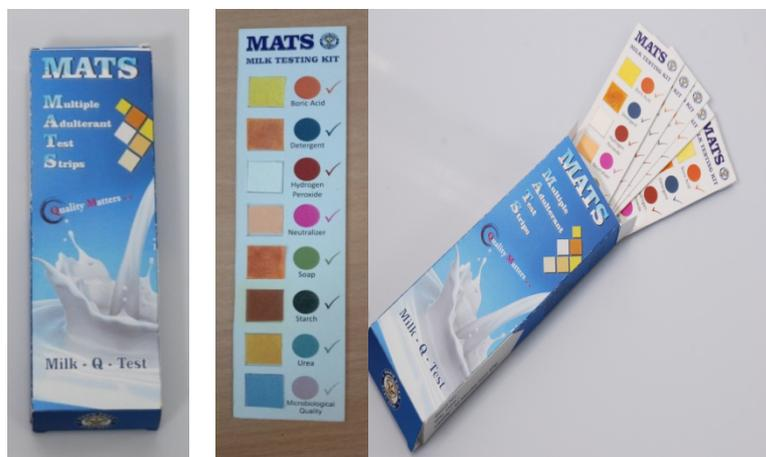
Mark II test kit has been envisaged as a portable, light weight, convenient, cost effective kit for popular household testing of milk quality, to make acceptance or rejection decision within 5 minutes.
