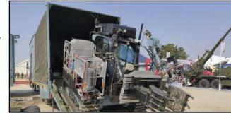
manipulator arm with a 3-axis cutting mechanism that holds the cutting nozzle of an abrasive water jet cutting machine for in-situ munition 'case entry'.
