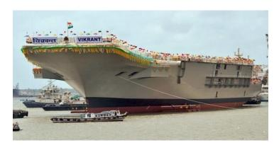
Plates of DMR249B have been used for the flight deck of the First Indigenous Aircraft Carrier (IAC), INS Vikrant
