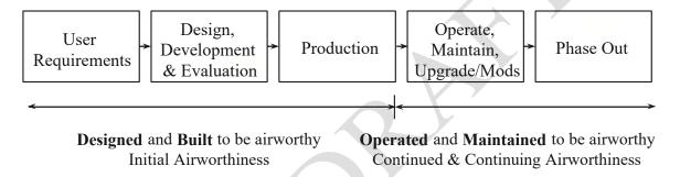
Figure 1: Airworthiness Concept during Air System Life Cycle
