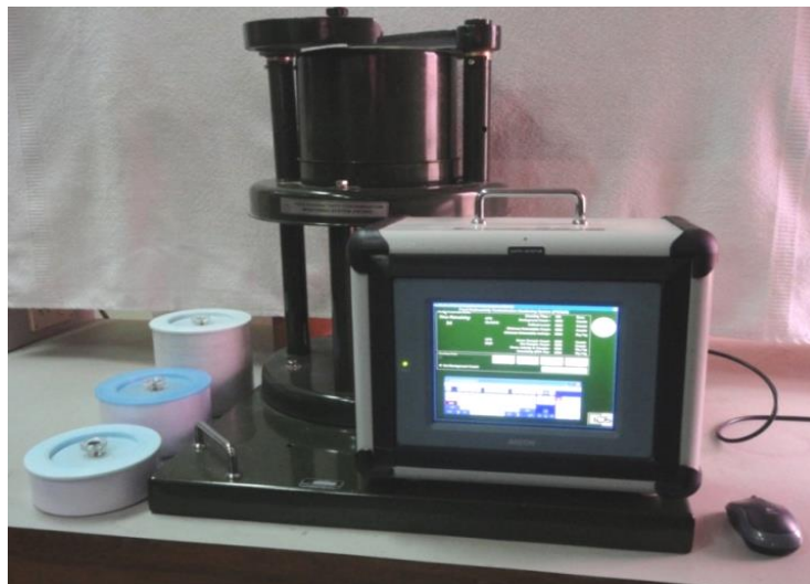
Fig 1: Food Radioactivity Contamination Monitoring System (FRCMS)
