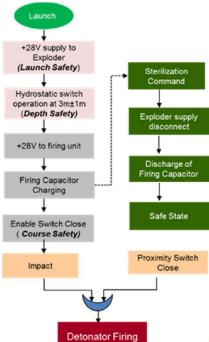
Fig 1: Exploder Sequence of Operations
