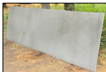
Indigenized AA2519-T87 plate (t = 15 mm)
