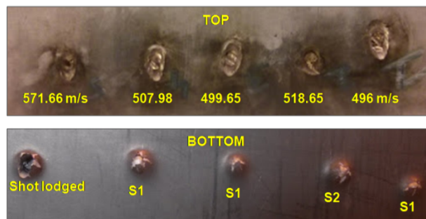
Top and bottom sides of the 15 mm thick AA2519-T87 plate subjected to the ballistic test against 7.62 x 54 mm AP (I) ammunition
