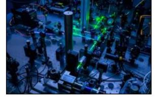
Amplified frequency-domain thermoreflectance setup used to study the existence of second sound in germanium. Two different lasers are focused onto the surface of the samples using a microscope objective. A rather large combination of optical elements allows to control and modify the spot size and shape, as well as the power and harmonic modulation of the lasers. Cold nitrogen gas is used for better visualization of the lasers optical path. Credit: ICMAB, CSIC
