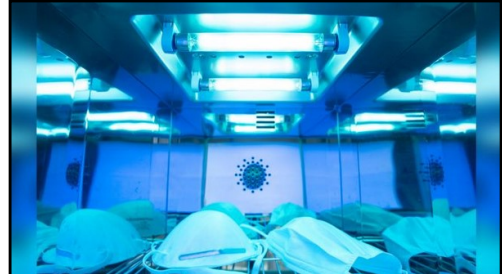
A handful of N95 respirators get zapped with UV radiation.
