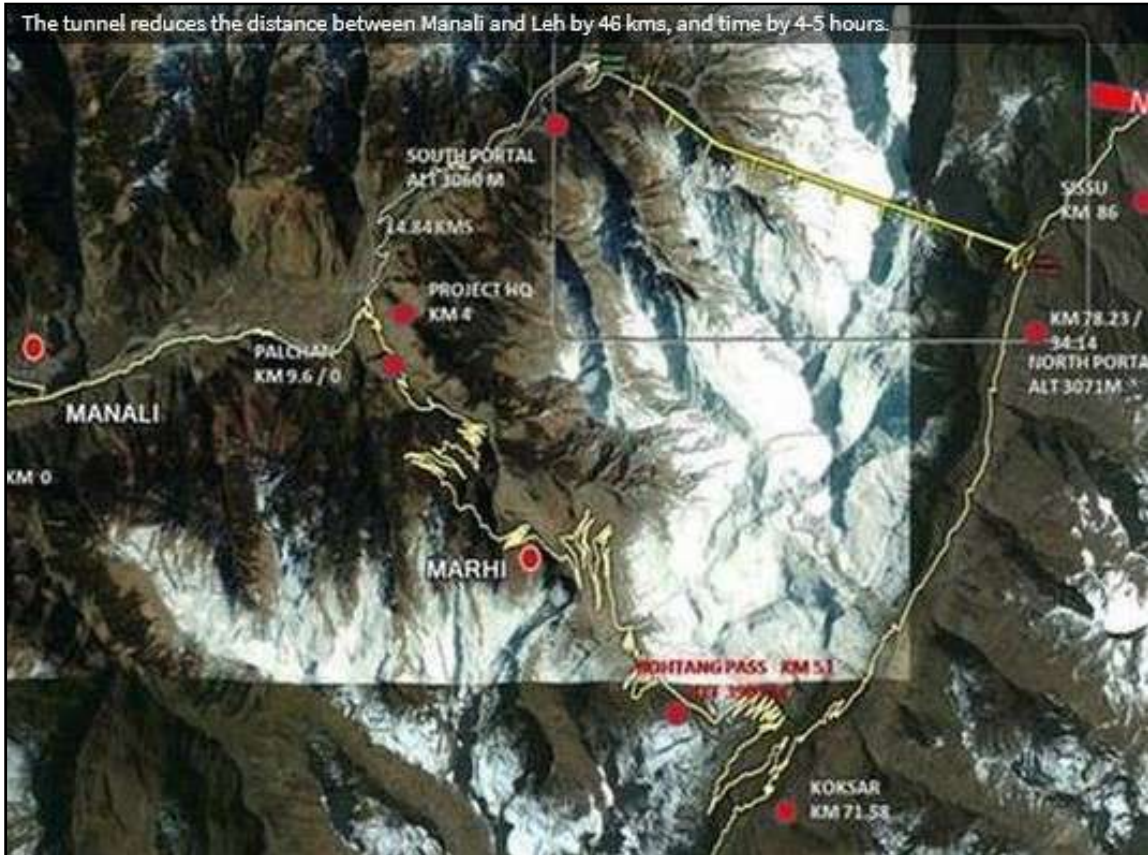
The tunnel reduces the distance between Manali and Leh by 46 kms, and time by 4-5 hours.
