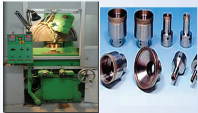
Curve Generation Machine and Diamond Tools
