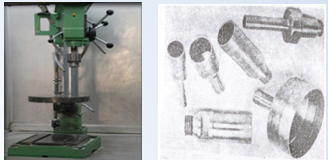
Trepanning Machine and Tools
