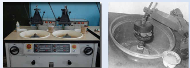
Grinding/Smoothing Machine and Smoothing of a Block
