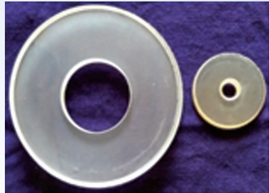
Polished Annular Obscured Aspheric Mirror
