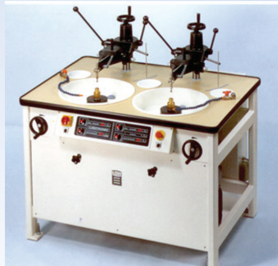
Loose Abrasive Grinding and Soothing Machine
