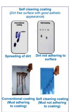
comprises hydrophobic PDMS epoxy resin, which resin and provide anticorrosive and self cleaning properties in a single coat application. The hydrophobic top surface ensures self cleaning of dirt and contaminants, while the epoxy layer underneath provides anticorrosive properties and excellent adhesion to metallic substrates. This coating can be applied on superstructure and interior compartments of ships as well as for multifarious civilian applications.
