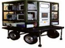
Skid mounted 10 kW PAFC
