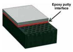
Schematic of tile-metal adhesion with epoxy putty
