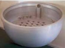
Torpedo node cone made of Aluminium alloys metal matrix components
