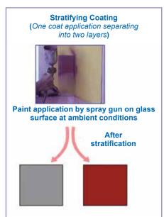
coatings facilitate segregation of two distinct interconnected coating layers with complimentary properties in a single shot application thus obviating the need of multiple coating steps.
