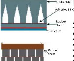
Schematic of the application of NMR51K and NMR88C adhesives
