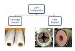
Cartridge loaded and case bonded grains
