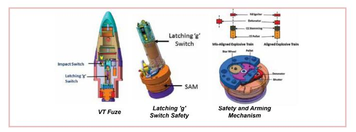
star wheel, gear, pinion and pallet mechanism. The detonator inside shutter comes to the armed position slowly. The motion of shutter is continuously hindered by the pallet and therefore it takes time (about 900 ms-1 s) for the detonator to come to aligned condition.
