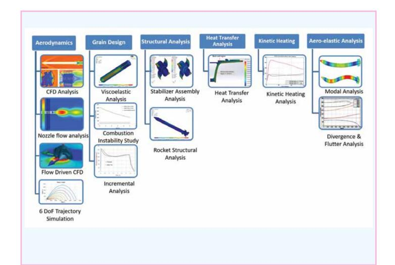
Simulation Techniques used in Design of Artillery Rockets
