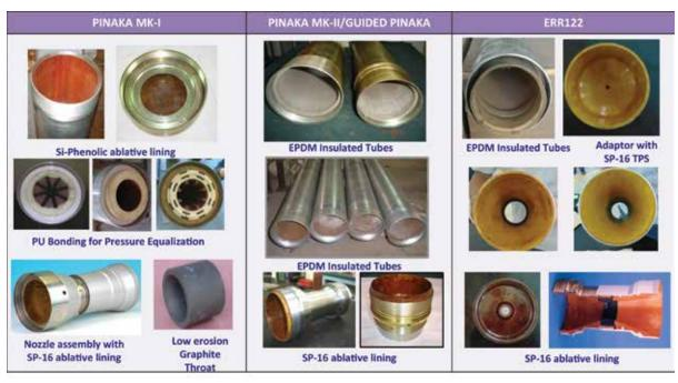
Thermal Protection System used for Rockets
