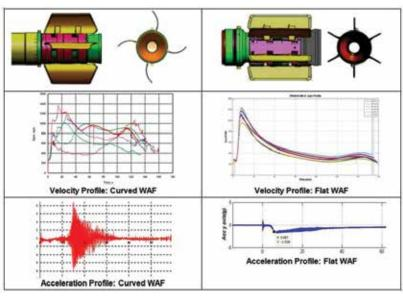
Stabilizer Redesign to Overcome High Mach Number Dynamic Instabilities (from curved Wrap Around Fin to Flat Wrap Around Fin stabilizer)
