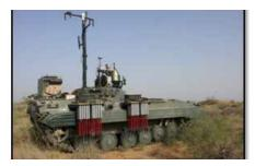
processes the sensor data to perceive its environment and react accordingly. Since it is a BMP-II vehicle with armor and tracked locomotion capability, it is the most suitable unmanned robot to carry out surveillance and reconnaissance in battlefields. The user can command it to continuously patrol or reach a spot on a map, and the vehicle can autonomously navigate, avoiding obstacles on its path, until it reaches its goal.
