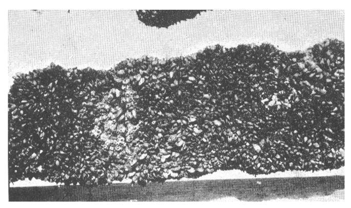
In a dry dock, the bottom of a ship can be cleaned of the entire mussel fouling but the byssal threads remain on the surface. Cleaning up of these flexible byssal threads is the nightmare of the workforce employed for the job.
