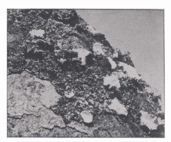
Fig. 3 : A portion of marker buoy showing extensive fouling
