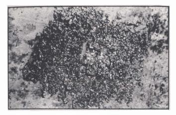
Fig. 4 : Seawater inlet blocked by mussel fouling
