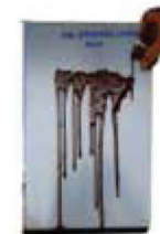
Conventional coating (Mud adhering to coating)
