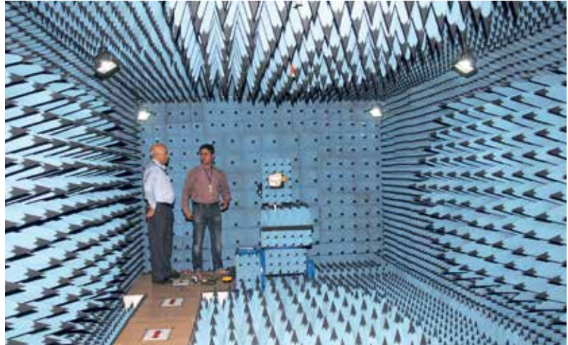
Far-Field Rectangular RF Anechoic Chamber
