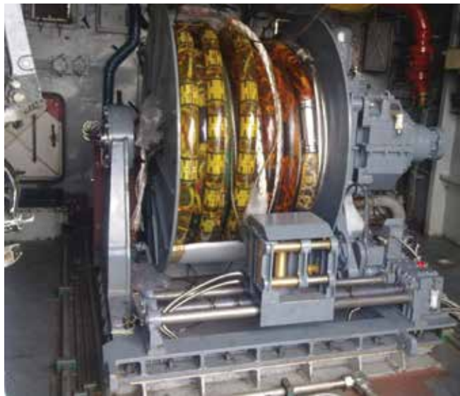
Maareech sonar processing system and winch with towed array onboard IN platform
