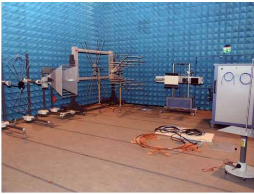
RF shielded Semi-Anechoic Chamber of the EMI/EMC Test Facility
