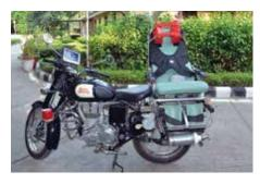
from low intensity conflict areas. This will be handy in the congested streets and remote locations, where access through ambulance is difficult and time consuming. The bike can respond to a medical emergency faster than a four-wheeler due to its functionality and integrated emergency medical support system. Rakshita is fitted with a customized reclining
