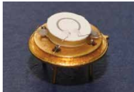
Prototype of Zirconia Amperometric Oxygen Sensor
