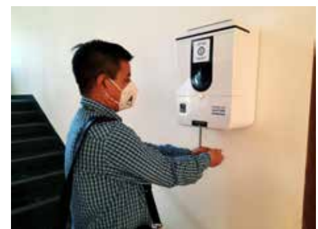
Automatic Mist Based Sanitizer Dispensing Unit
