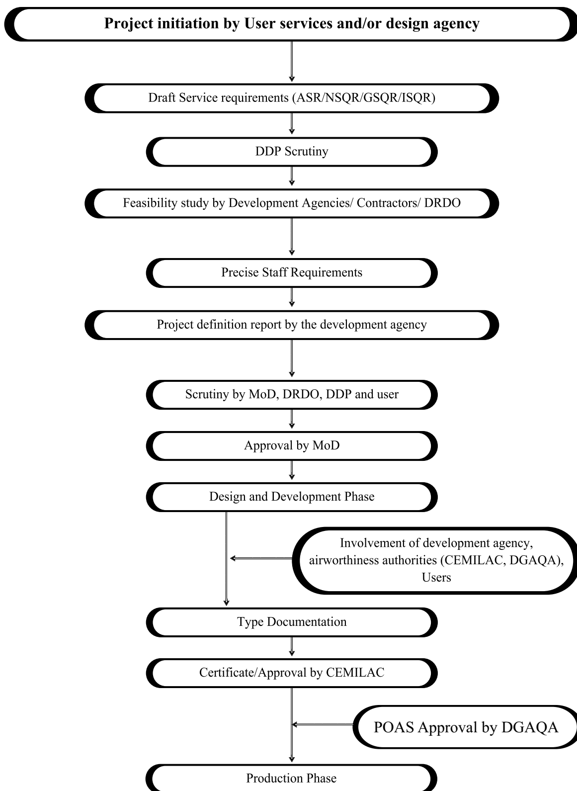
Figure A.1 Procedure for Project initiation & development
