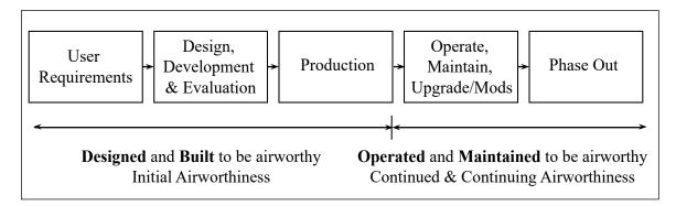
Figure 1: Airworthiness Concept during Air System Life Cycle
