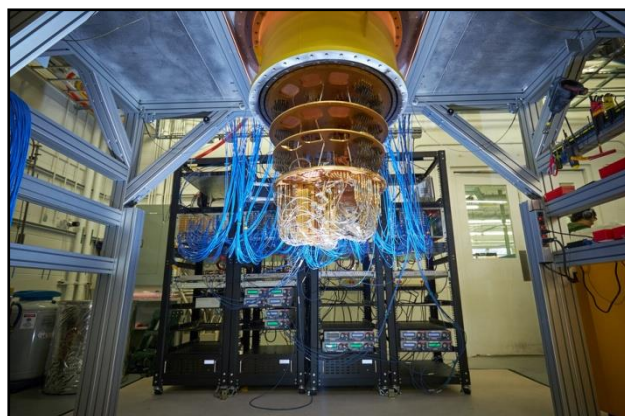
Google's Sycamore processor mounted in a cryostat, recently used to demonstrate quantum supremacy and the largest quantum chemistry simulation on a quantum computer. Credit: Rocco Ceselin
