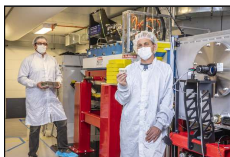
Sam Barber, left, a research scientist at Berkeley Lab's BELLA Center, and Jeroen van Tilborg, a staff scientist at the BELLA Center, hold the active plasma lens, right, and dipole magnets used in an electron-beam diagnostic experiment. The setup enabled measurements of electron-beam energy, with range and resolution comparable to what is achieved using the multi-ton magnet located behind them. Credit: Marilyn Sargent/Lawrence Berkeley National Laboratory
