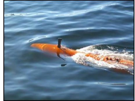
Kongsberg Maritime's HUGIN AUV is a powerful tool for deep-water hydrographic surveys. Photo: Kongsberg
