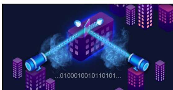
A concept figure of the MDI-QKD experiment in a city. Telescopes are located in high-rise buildings for transmitting encoded photons. The turbulence of the atmosphere, which exists everywhere in the transmission channel, is the main challenge for the photons to maintain the spatial mode in the detection terminal. Credit: Yao Zheng/Micius Salon.
