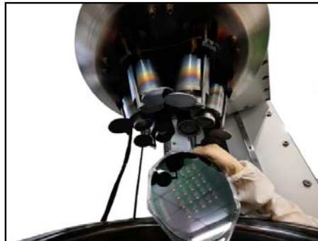
The sputtering technique has been widely used for thin film deposition. Under the sputtering guns, an eight-inch wafer with patterned device fabricated by deposition, photolithography, etching, etc. is shown. Credit: NTHU MSE, Taiwan
