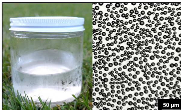
Photo shows water microdroplet condensate formed on the surface of a glass container containing cold water (left) and an image of water microdroplets formed on a polished silicon surface (right). Credit: Jae Kyoo Lee and Hyun Soo Han
