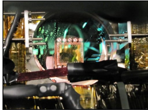
A look at the atom chip in the experimental setup. Credit: Vienna University of Technology
