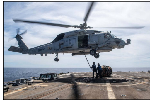
U.S. sailors assigned to the guided-missile destroyer USS Truxtun (DDG 103) conduct a simulated vertical replenishment with an MH-60R Sea Hawk helicopter attached to the Swamp Foxes of Helicopter Maritime Strike Squadron (HSM) 74, April 28, 2020. (Picture Source U.S. Navy)
