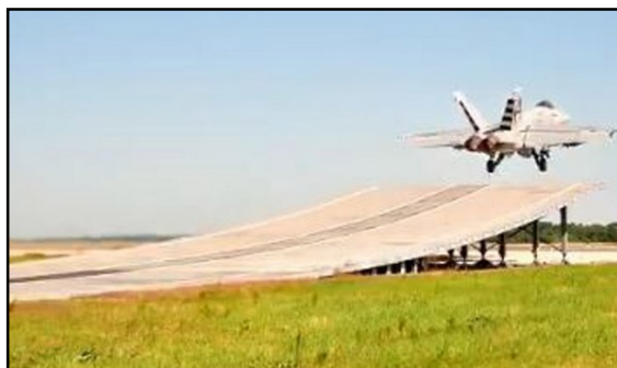
A Super Hornet taking off from a ski-jump | Twitter handle of Boeing
