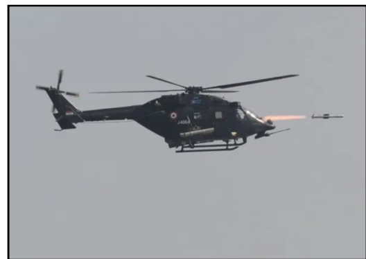
HELINA (Helicopter based NAG) is mounted on the Advanced Light Helicopter ( www.drdo.gov.in )
