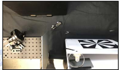
Setup of the experiment, new camera with polarizer on the left, hidden image, in this case a black-and-white pinwheel image, on the right.
