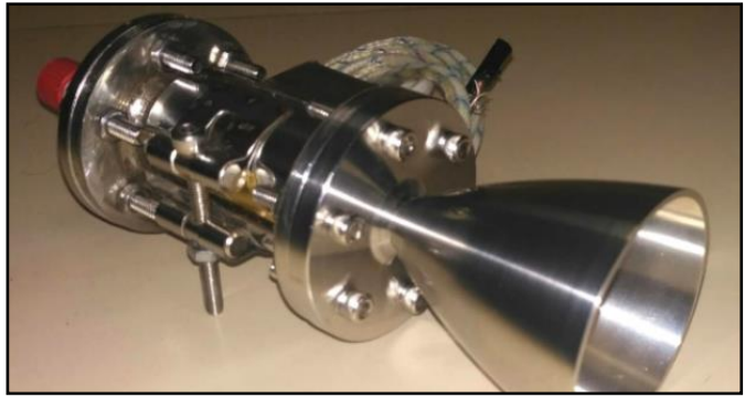
I-Booster thruster developed by Manastu Space Technologies Pvt Ltd
