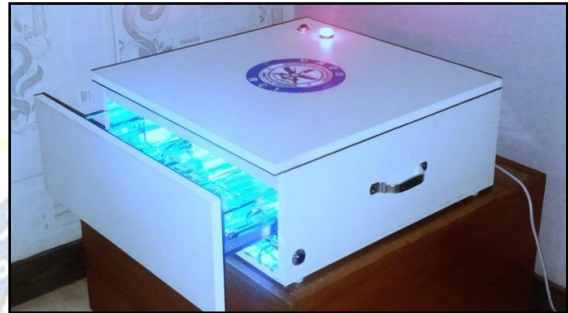
Disinfection tray developed by Hyderabad's lab to sanitise currency notes, mobile phones etc.
