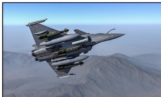
A Rafale flying with three 1,000kg AASM HAMMER weapons | © ERIDIA Studio via Dassault Aviation
