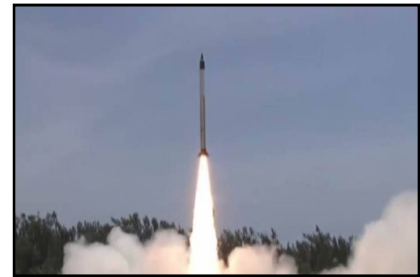
The HSTDV will comprise of a solid rocket component to get it into the air and flying and subsequently it will utilize its scramjet engine to rise and accelerate to a high elevation where its jet engine functions most proficiently. (Photo source: Video screengrab)
